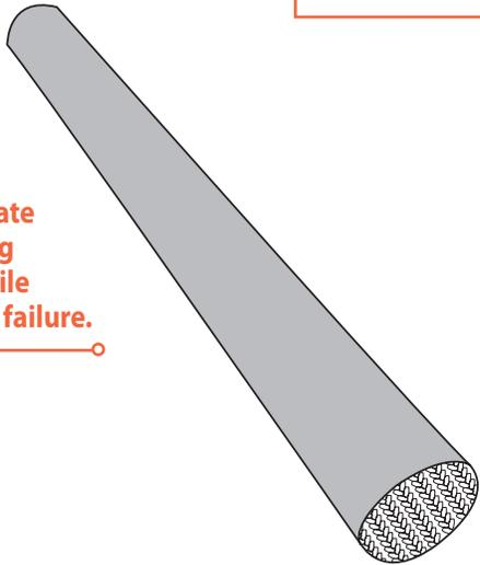
When applied, the aluminum laminate reflects heat away and the insulating fiberglass backing protects the fragile contents from thermal damage and failure.
