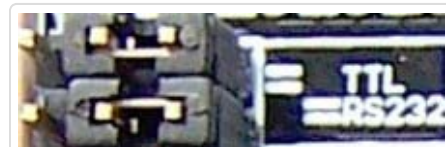
(/wiki/index.php/File:Sdb_v2.2_5.pr RS232/TTL Selection Jumpers
