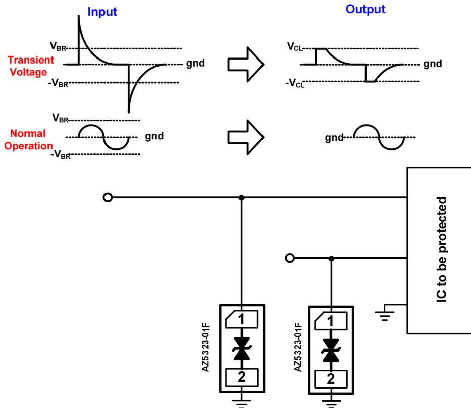
Fig. 1 ESD protection scheme by using AZ5323-01F.
