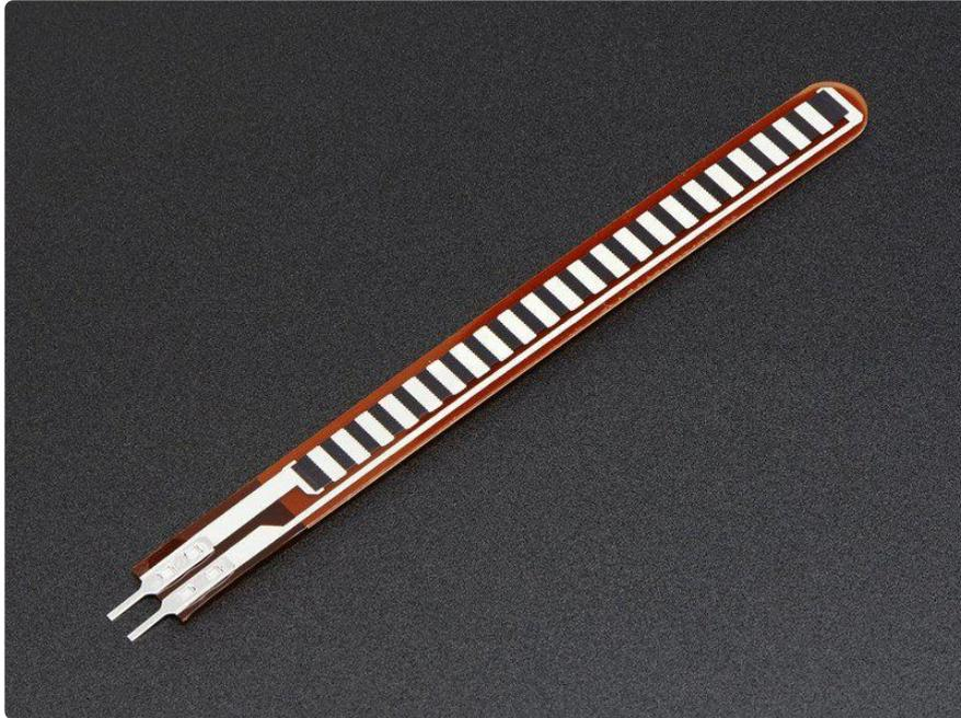
This sensor can detect flexing or bending in one direction. They were popularized by being used in the Nintendo PowerGlove as a gaming interface.
