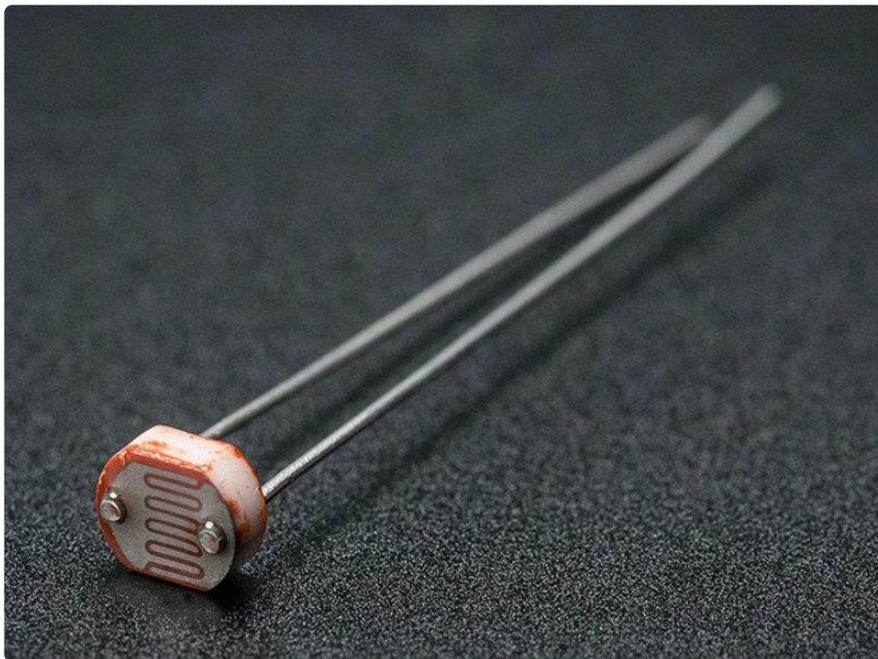
Photocells are sensors that allow you to detect light. They are small, inexpensive, low-power, easy to use and don't wear out. For that reason they often appear in toys, gadgets and appliances. They are often referred to as CdS cells (they are made of Cadmium-Sulfide), light-dependent resistors (LDR), and photoresistors.
