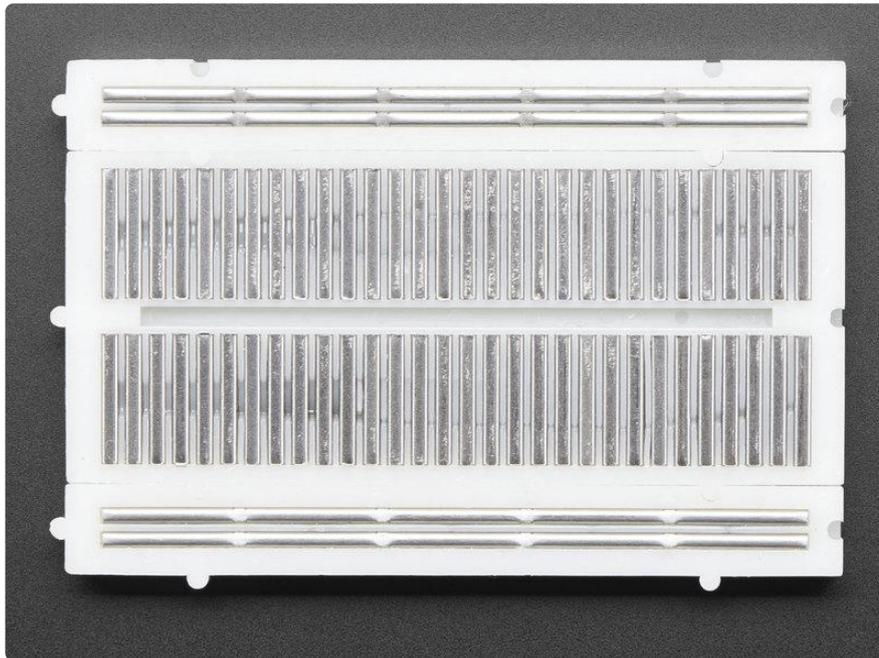
If you pulled the metal parts out with pliers (again, don't do this yourself!) You'd see each one is a metal clip with little teeth. The rows have 5 teeth - one for each hole on the top of the breadboard. (The power rails have 50 teeth)
