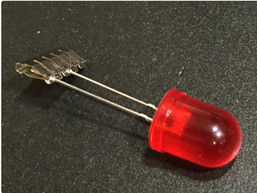
Each clip can handle at least a hundred plugs and unplugs before the springiness of the clip slowly weakens and eventually stops gripping so well. You'll know when the breadboard needs replacing because you won't feel the clip gripping onto the part when you press it in.
