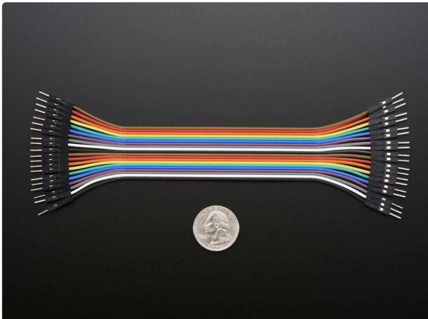
Each version comes in a 'strip' of 20 (2 pieces of each of ten rainbow colors). They have 0.1" male header contacts on either end and fit cleanly next to each other on standard-pitch 0.1" (2.54mm) breadboards. The best part is they come in a 20-pin
