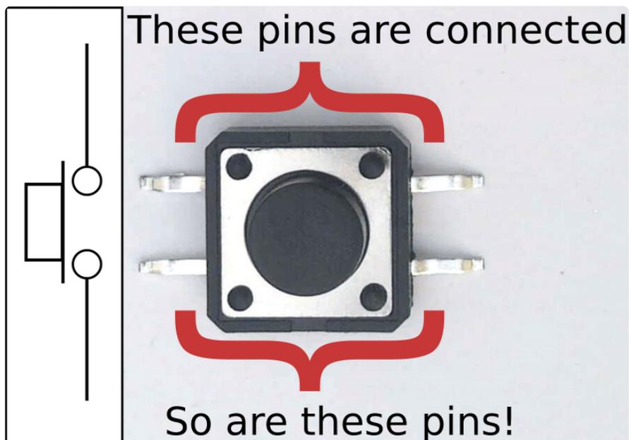
So don't forget when using in the breadboard that the two rows across from each other will be connected on the inside of the switch!
