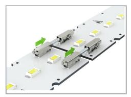
Assembly: Place PCBs on a flat surface and insert links into terminal blocks on adjoining PCBs. Disassembly: Open the terminal blocks with an operating tool. (max. 5 connections /disconnections)
