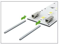
Insert the board-to-board links into the terminal blocks.
