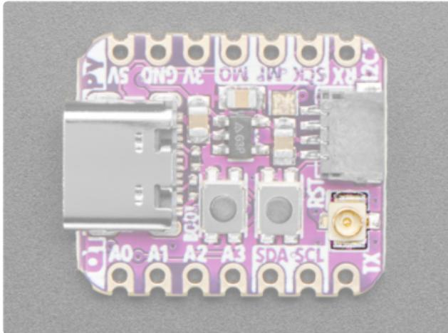
The [Adafruit QT Py ESP32-S2 WiFi Dev Board with uFL Antenna Port](#) () comes with, you guessed it, a uFL antenna port! This is the only version that has the port!
