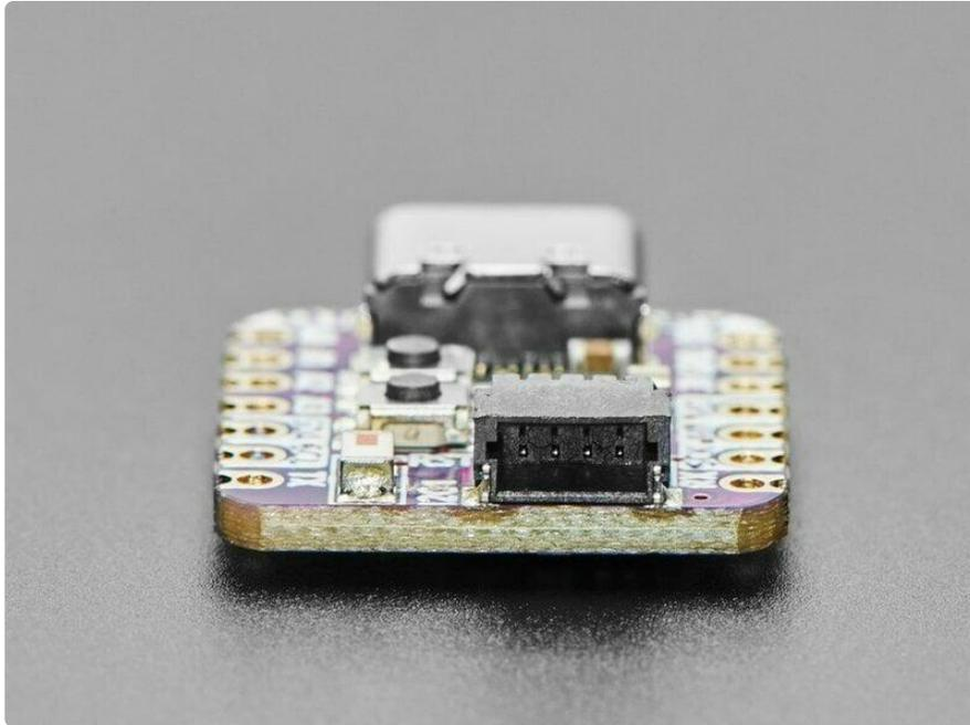
Pinout and shape are [Seeed Xiao \(\)](#) compatible, with castellated pads. In addition to the QT connector, we also added an RGB NeoPixel (with controllable power pin to allow for ultra-low-power usage), a reset button (great for restarting your program or entering the bootloader) and a button on GPIO 0 for entering the ROM bootloader or for user input
