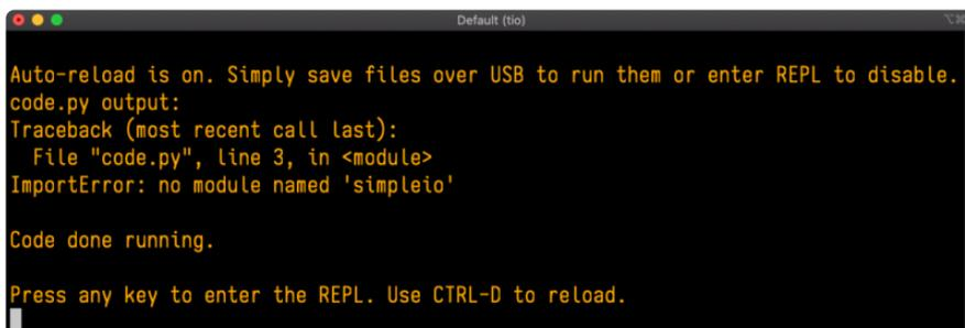
A screenshot of a terminal window titled "Default (tio)". The terminal output shows a message about auto-reload, followed by a traceback indicating an ImportError: no module named 'simpleio' at line 3 of 'code.py'. The terminal also shows "Code done running." and a prompt to press any key to enter the REPL.
