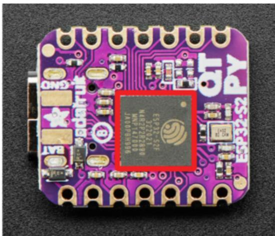
The ESP32-S2 microcontroller (highlighted in red) is located in the center of the back of the QT Py.
