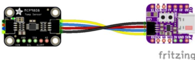
Simply connect the STEMMA QT cable from the STEMMA QT port on your board to the STEMMA QT port on the MCP9808.
