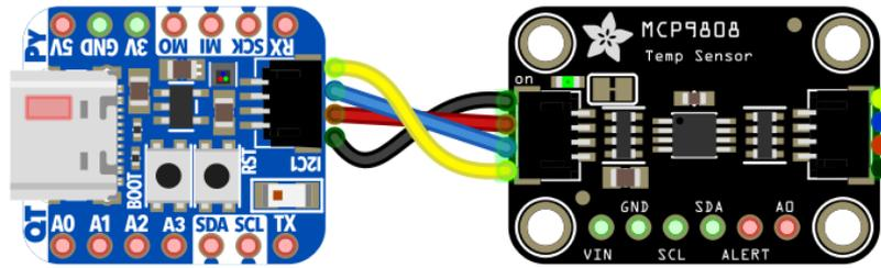
Note we are using the STEMMA QT port here, that means we need to reference Wire1 for I2C communication and also add `Wire1.setPins(SDA1, SCL1)` in our code in setup()
