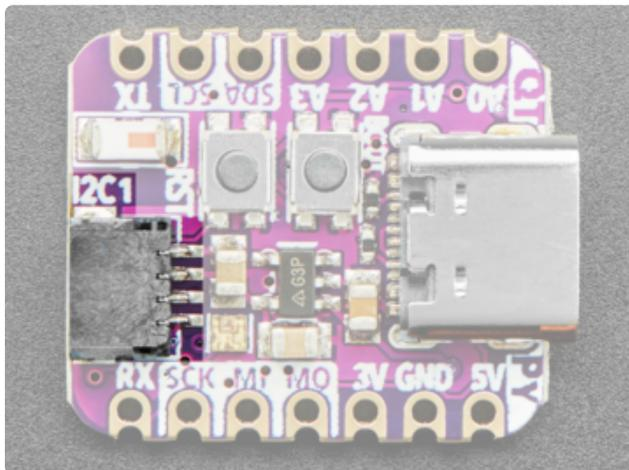
The QT Py ESP32-S2 has TWO I2C ports!
