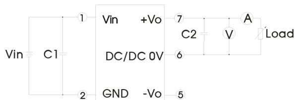
Note: C1,C2,C3: 100uF/35V (Low internal resistance capacitance)
